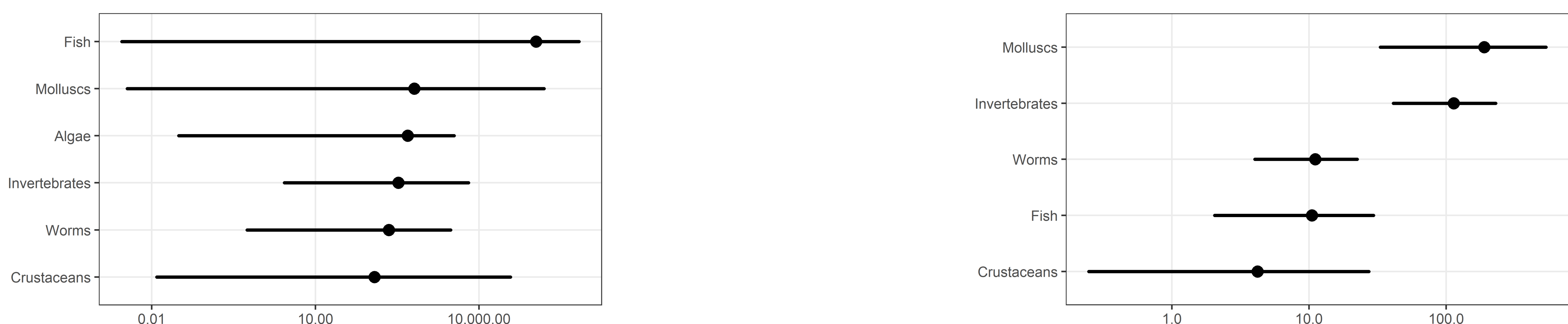
Figure 2. Cumulative risk quotients (weighted average and 95% CI) for a contaminant mixture in stormwater entering the Oslofjord. The figures display predicted acute (left) and chronic (right) toxicity to different organism groups.
