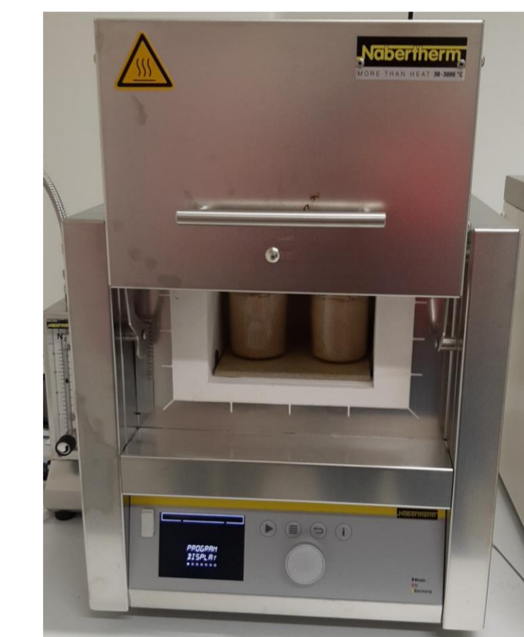
Preparation of sediment test materials for the ILC. Cleaned in an oven, and ready to be spiked with polymers.
