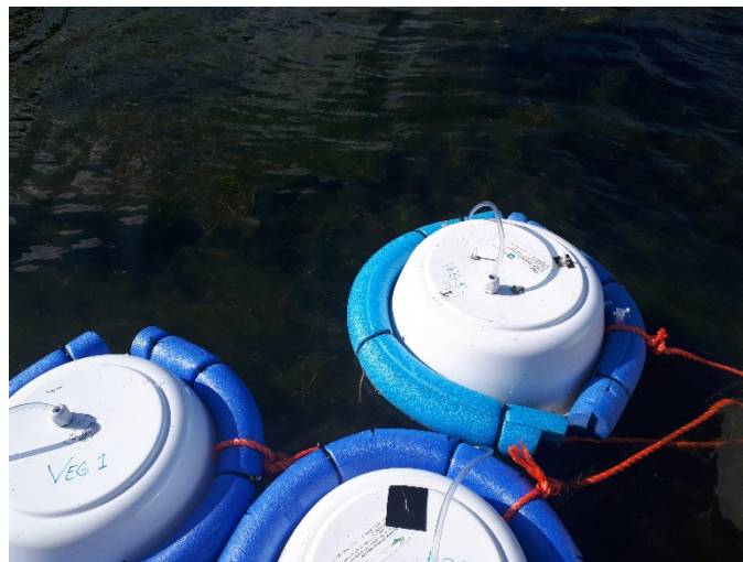
Fig. 5: Floating chambers to measure greenhouse gas emissions in Lake Kemnade in July 2020
