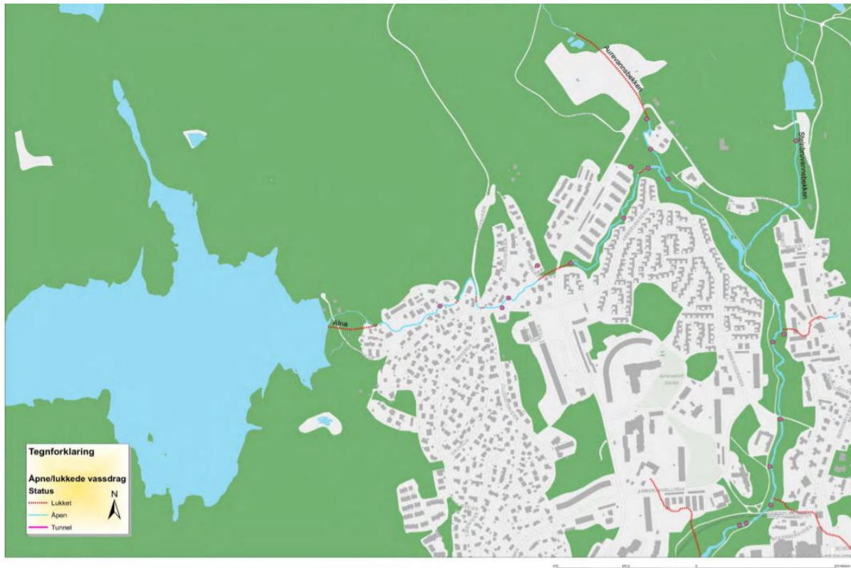
Fig. 3: Source of the Alna at Alnsjøen lake in the north-east of Oslo. Red dashed lines indicate piped sections of the river, blue signals open sections and dots denote point-source pollution. At the top of the map shows the Aurevannsbekken tributary passing under Huken quarry (Source: NIVA, 2020).
