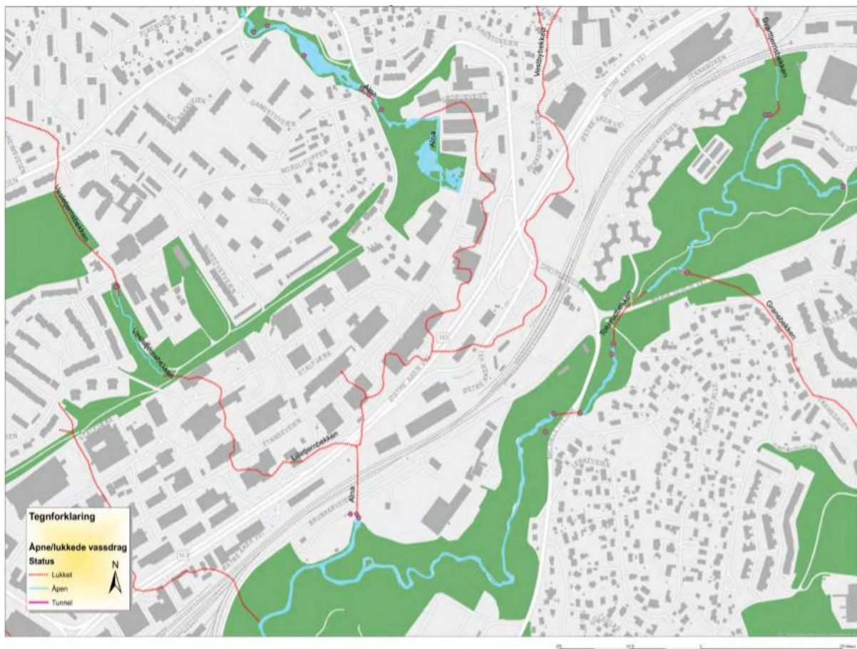
Fig. 4: Map of the subregion around the Grorud train station. Dots indicate point-source pollution, red dashed lines show closed sections of watercourses, with blue showing open watercourses. Hølaløkka park is present in the upper-middle of this map (Source: NIVA, 2020).
