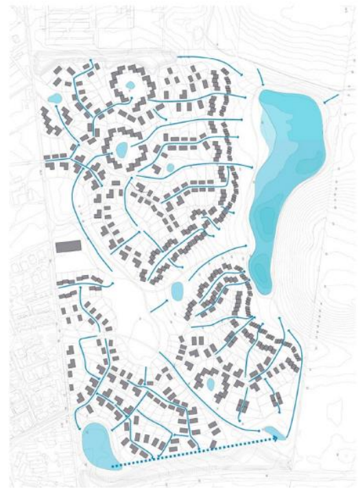
Figure 17: In the Bellinge Fælled district area, rainwater is handled within the district (Odense Kommune, 2013)
