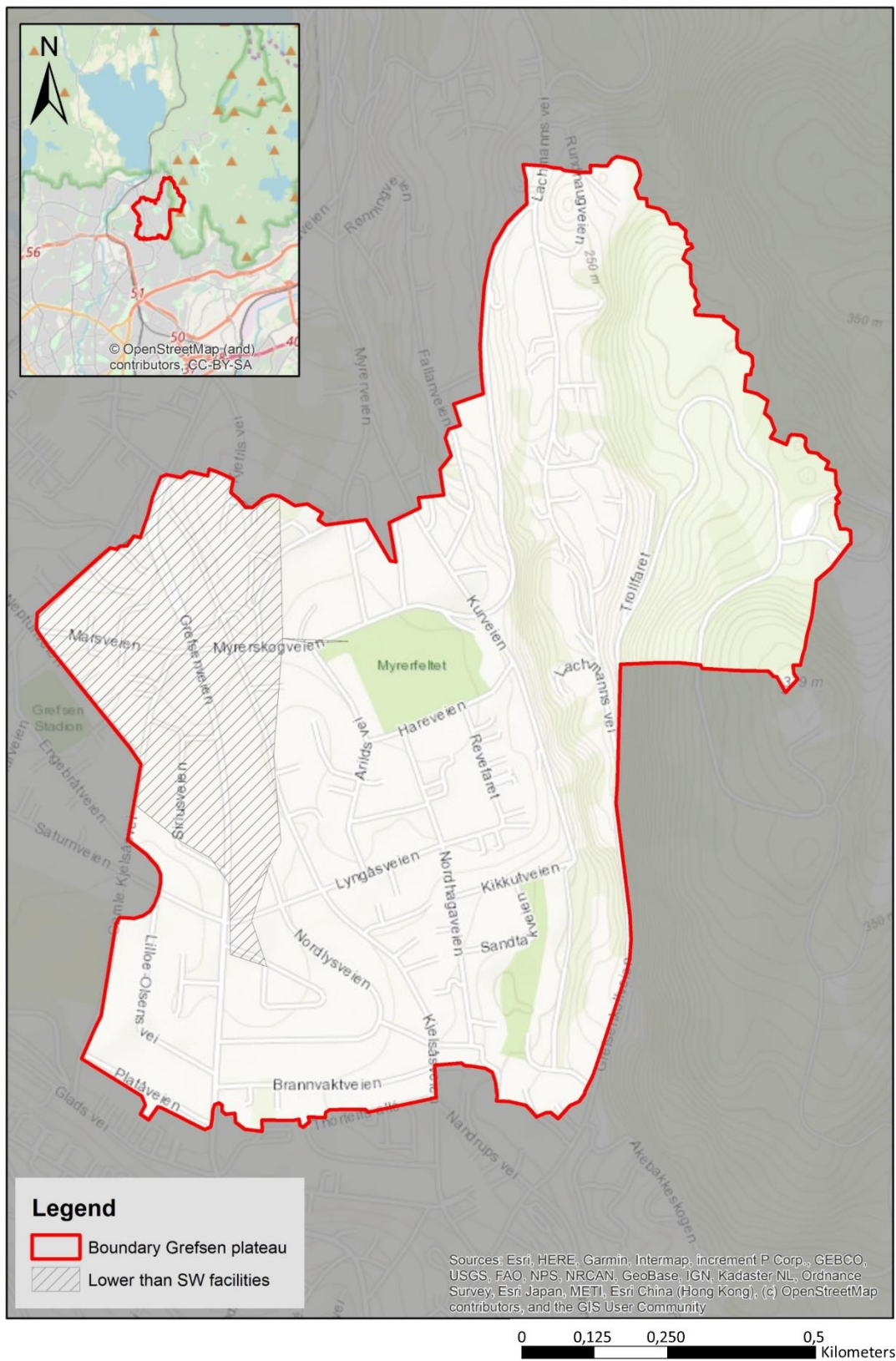
Figure 19. approximately 15 % of Grefsen has a lower elevation than potential implementation locations for large scale wadis or water squares.
