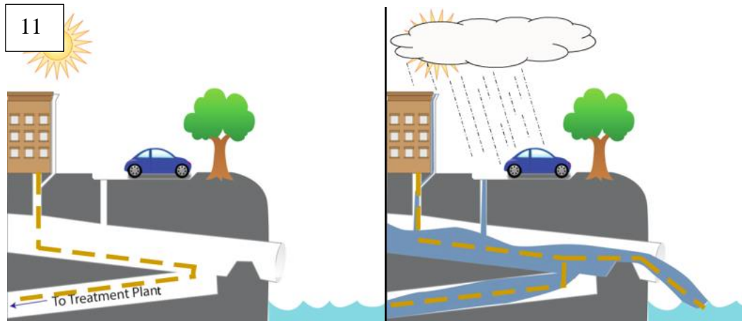
Figure 16. Combined sewer system
