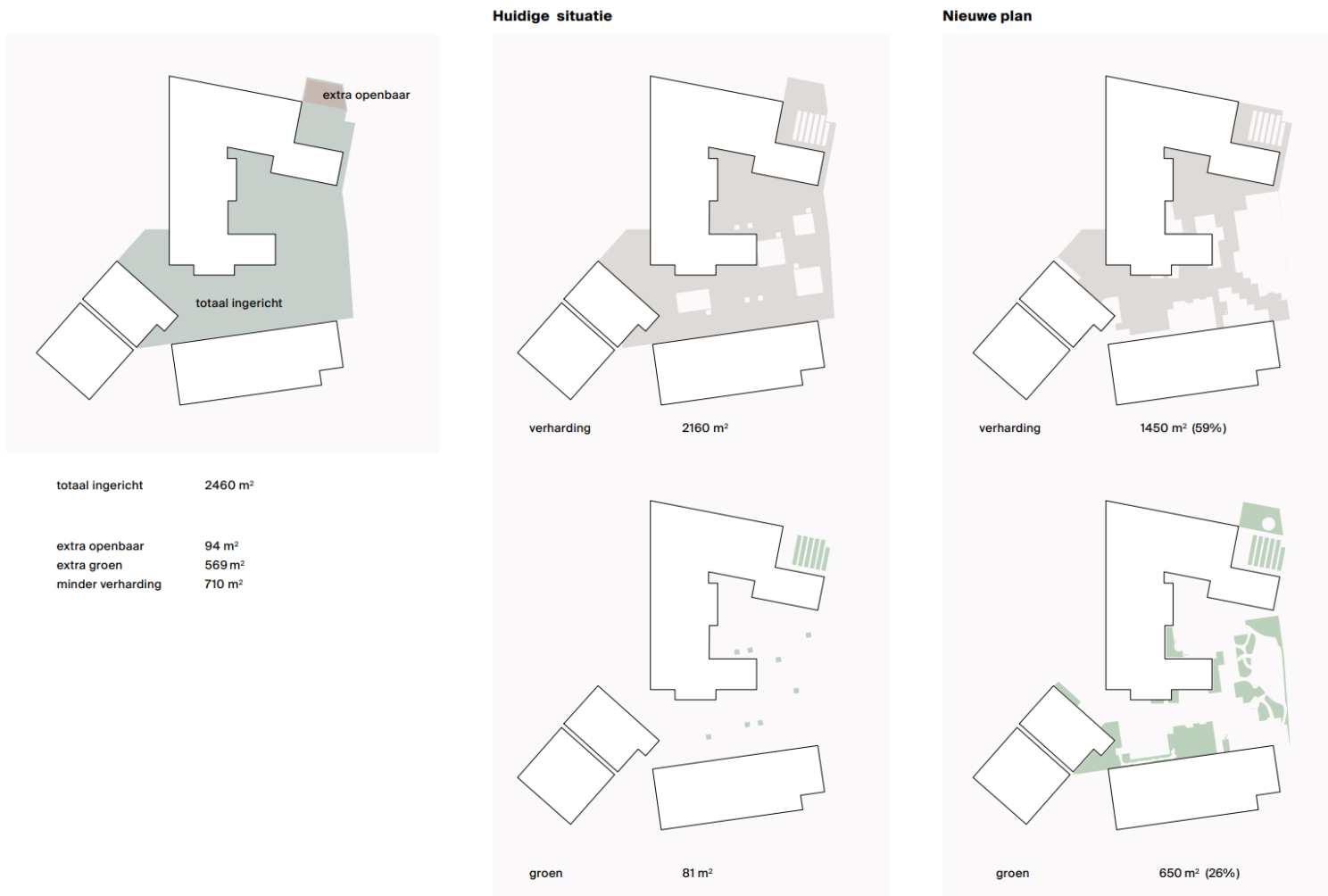
Figure 15. De Ijsbreker's surfaces of the baseline (huidige situatie) and new design (nieuwe plan) schoolyards of the elementary school De Ijsbreker
